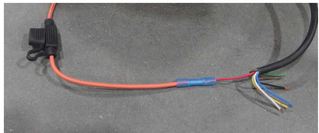
Red wire connects to the orange fuse wire.
